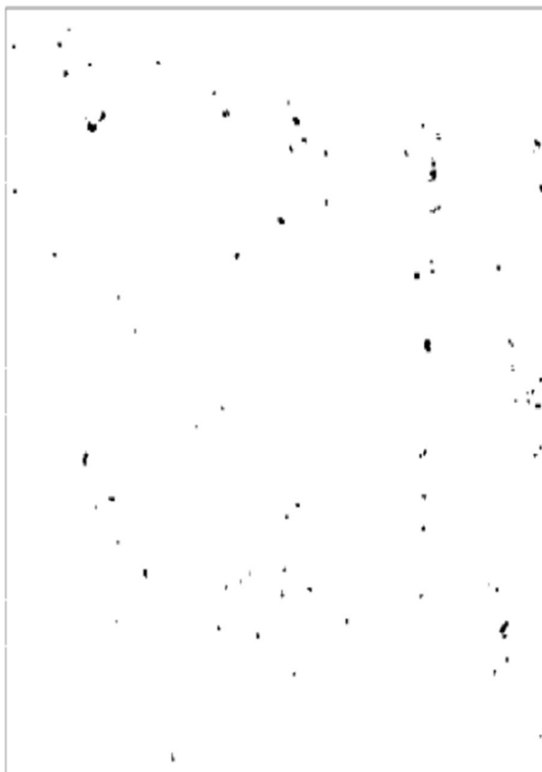
Figure A.2 — Degree of rusting R1.2
