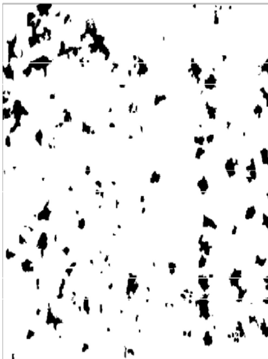
Figure A.4 — Degree of rusting DI 4
